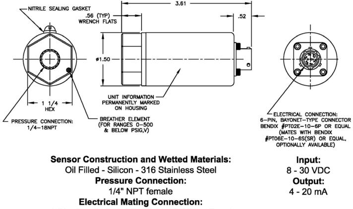
6-Pin, Bendix P/N: PT06E-10-6S(SR) or Equal
