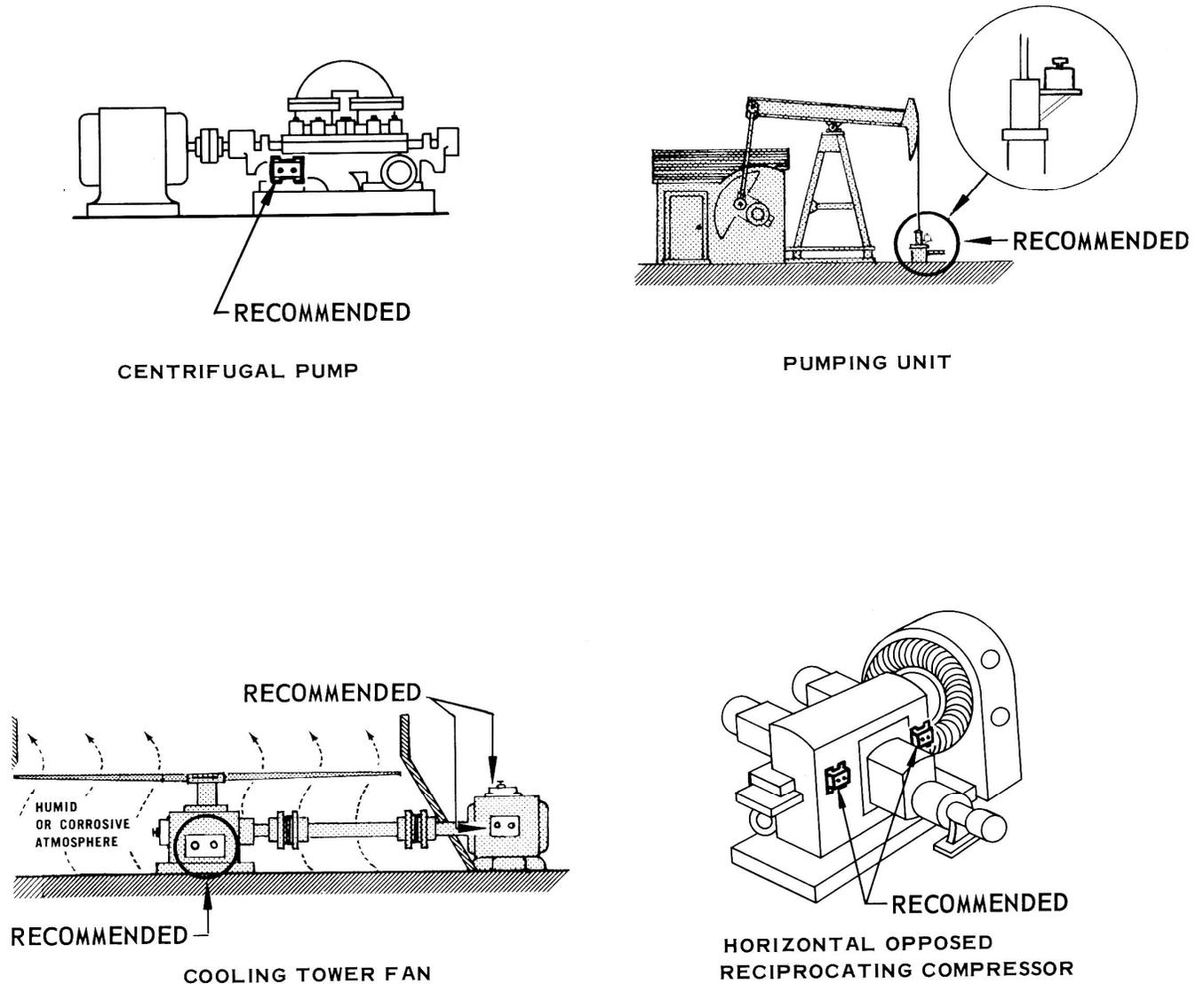
Figure 3-2, Methods of Mounting the Vibraswitch, Model 366. (Sheet 2 of 2).
