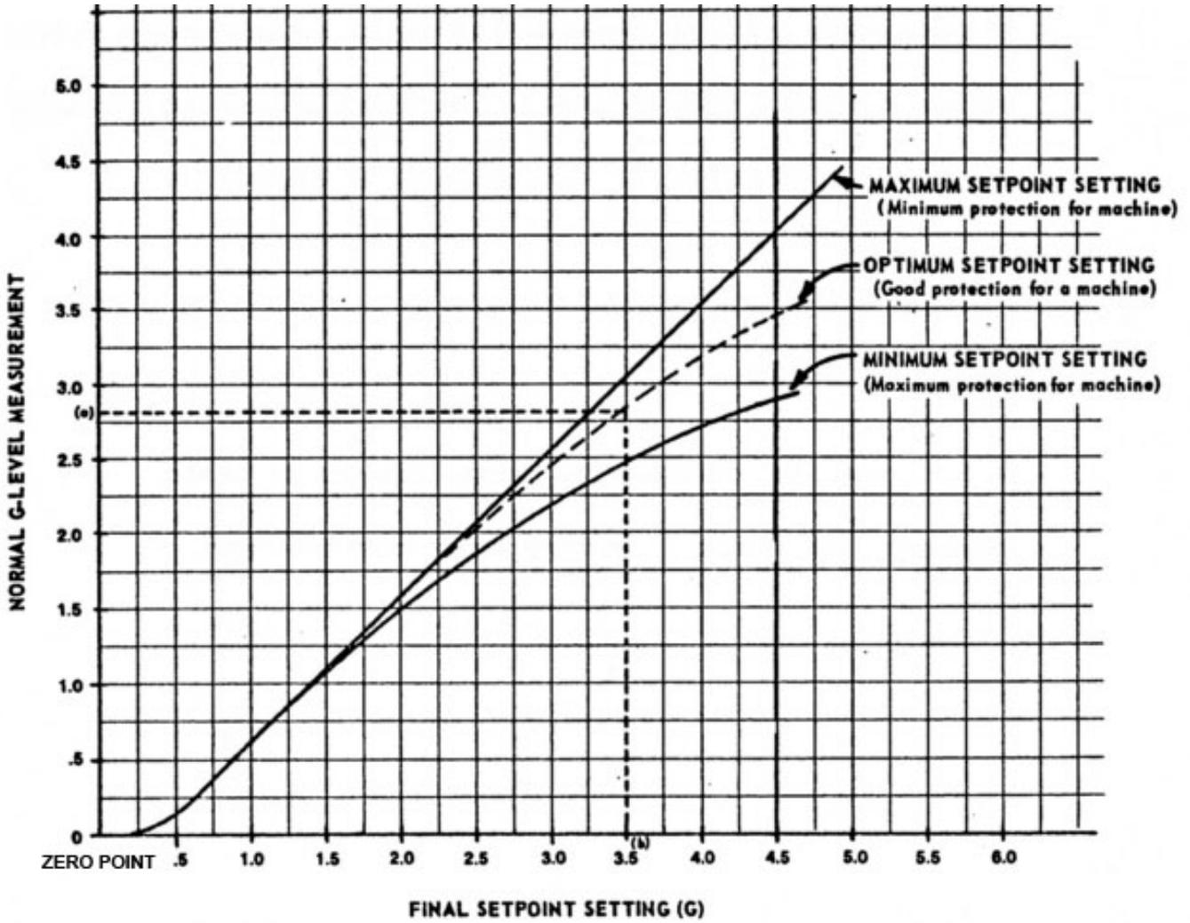
**EXAMPLE:** If the normal g-level (a) is 2.8 g above the Zero Vibration Level, the Final set point settings (b) should be set at 3.5 g above the Zero Vibration Level. Therefore, advance the set point pointer CCW .7 g ( $3.5g - 2.8g = .7g$ ) or 7 divisions (one scale division (one scale division is .1 g) from the normal g-level.
